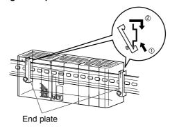
To fix CJ1 assembly securely, sandwitch the assembly using a pair of endplates from both sides. Fook lower notch of the end plate to the lower plate of the rail
