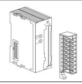
Terminal block can be detached by pulling down the lever. Normally, the lever should be in upper position.
