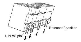
2. Hook the CJ unit's upper protrusions on the DIN rail ( 1 ), and engage the entire notch to the rail ( 2 ).
