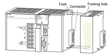
CJ series do not require base unit. Each unit can be connected to each other using the integrated side-mount connector.
