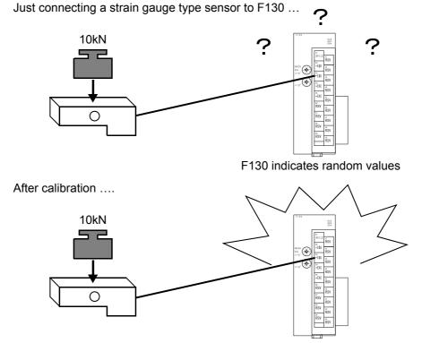
The F130 and strain gauge type sensor function as a weighing device
